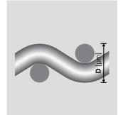
Mesh thickness **D** [μm] The mesh thickness **D** is measured according to DIN 53855-1. The tolerance is the defined range of the statistically ascertained mean values of mesh thickness.
