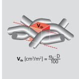
Theoretical ink volume  $V_{th}$  [cm³/m²] The theoretical ink volume  $V_{th}$  is calculated from the mesh thickness D and the percentage of open area  $\alpha_0$ .
