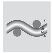
Mesh thickness D [ $\mu$ m] The mesh thickness D is measured according to DIN 53855-1.
