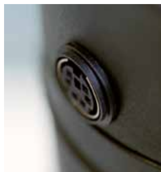
Interface serial RS 232 da SEFAR® Tensochek 100i
