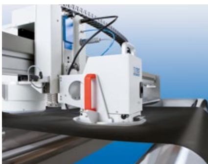
In-line testing of air permeability
