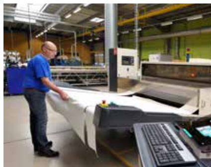
Fabrication – Laser cutting
